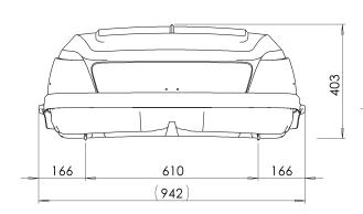
Note: \* Min distance between roof rails
